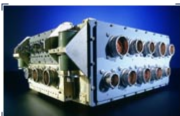
FADEC Hispano-Suiza (Boeing 777 explanation)
