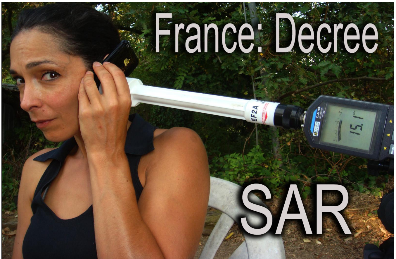
Isotropic fieldmeter reading of HF mobile phone radiation \leq 2.5 GHz ( 15 V/m = 60 \mu W/cm 2 ) – Photo Maya-Press EHS Gallery
