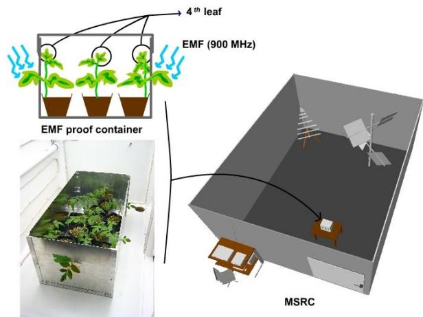
**Fig. 1. Experimental set up for shielding experiments.** Tomato plants (3-weeks old) are placed either totally inside an EMF-proof container (control plants) or with the 1st leaf left outside (exposed plants). After exposition to EMF, the 4th (protected) terminal leaf is collected for analysis.
